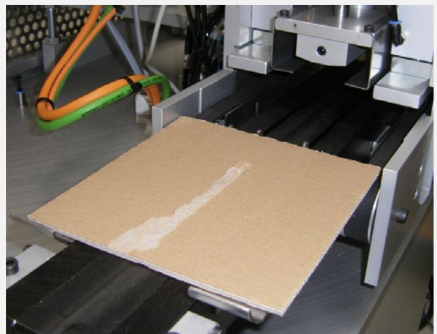
Ejection of the lower cardboard for visual examination.
